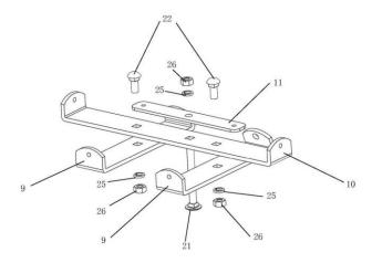
3. Attach Part A, Part B and Blade Bracket (#2) with 2pcs Carriage Bolt (#22), 2pcs Carriage Bolt (#23), 2pcs Flat Washer (#24), 4pcs Lock Washer (#25) and 4pcs Nut (#26) as Part C.
