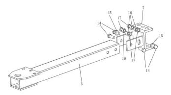
6. Finally attach Part C, Part D and Part E with Carriage Bolt (#18), Axle Pin (#19), Clip (#20), Lock Nut (#27) and Flat Washer (#28) together.
