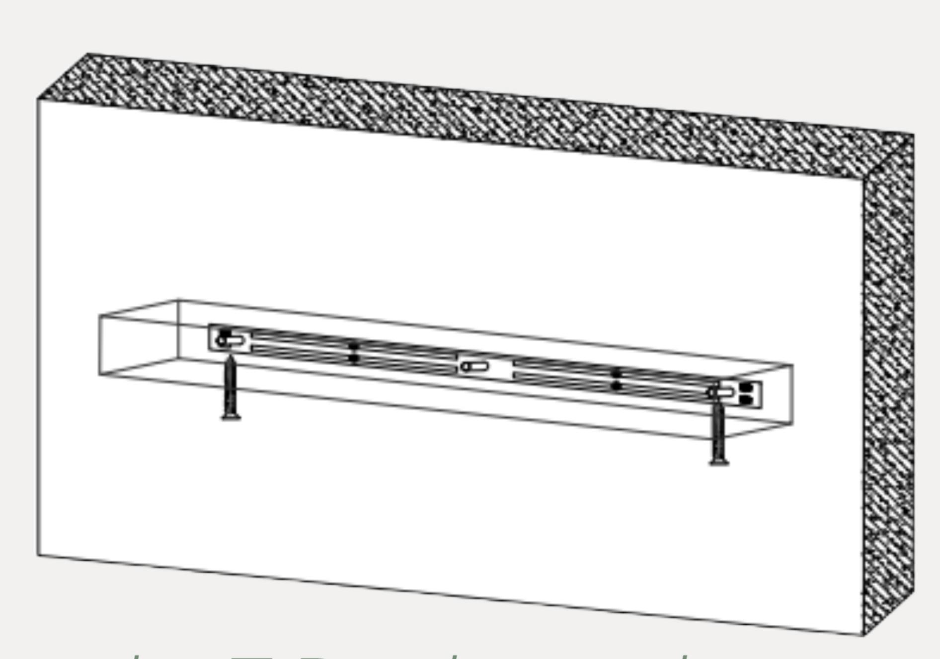
Step 5: Place the shelf/mantel onto the T-Bracket and reinstall set screws to ensure shelf cannot slide off bracket. (Set screws can be arranged to be on top or bottom of the shelf, arrange the layout in a way that works best for your application!)
