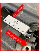
Mount the clip to a rib of the tailgate. Make sure the tube faces the passenger side of the truck. CAB arrows point to the front of the truck
