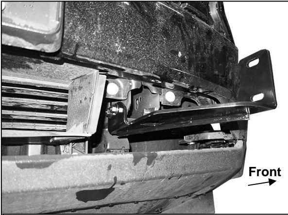
(Fig 12) Driver/left Bracket installed. NOTE: Center panel in bumper pictured removed for instruction purposes only
