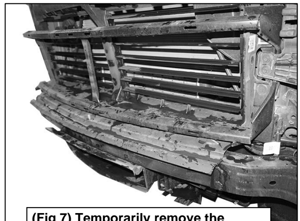
(Fig 7) Temporarily remove the plastic cover located below the grille
