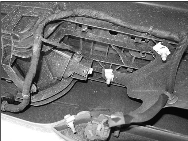
(Fig 5) Remove remote antenna (Fig 10), parking sensors and wiring harness as equipped
