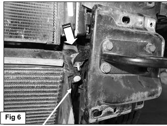
Diesel models, loosen top support bracket hardware at frame and intercooler (large arrow). Temporarily remove lower hanging intercooler bracket from side of frame
