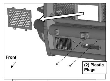
(Fig 18) Attach License Plate to Bumper
