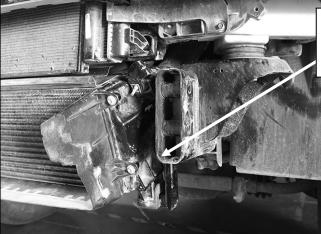
(Fig 7) Reinstall Intercooler brackets
