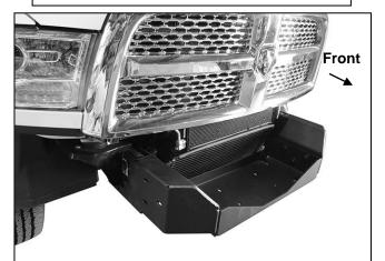
(Fig 12) Attach Winch Tray to Frame Brackets
