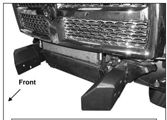
(Fig 10) Frame Mounting Brackets installed
