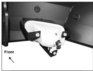
(Fig 19) Line up the tabs with the OE fog light if equipped. Carefully push the fog light into the mounting tabs
