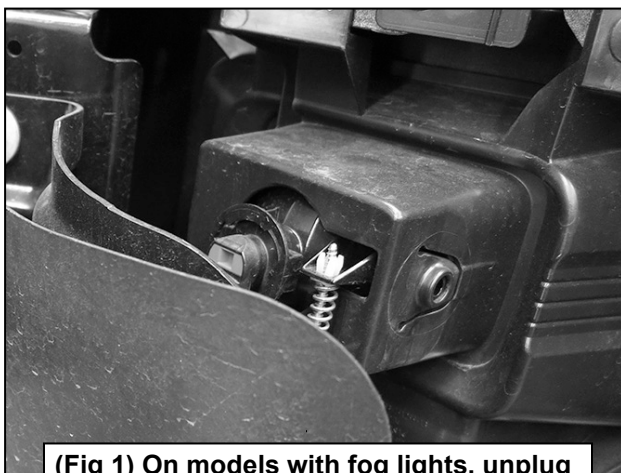
(Fig 1) On models with fog lights, unplug wire harness from back of light
