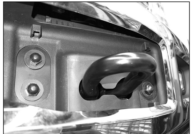
(Fig 6) Remove bumper bolts (driver side pictured)
