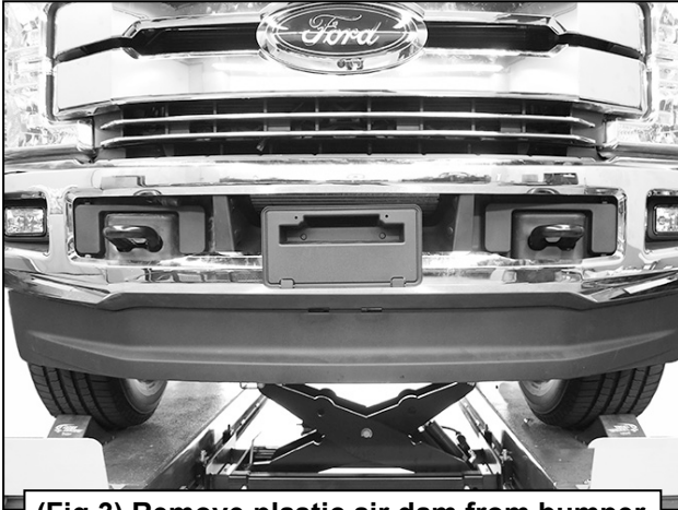
(Fig 3) Remove plastic air dam from bumper
