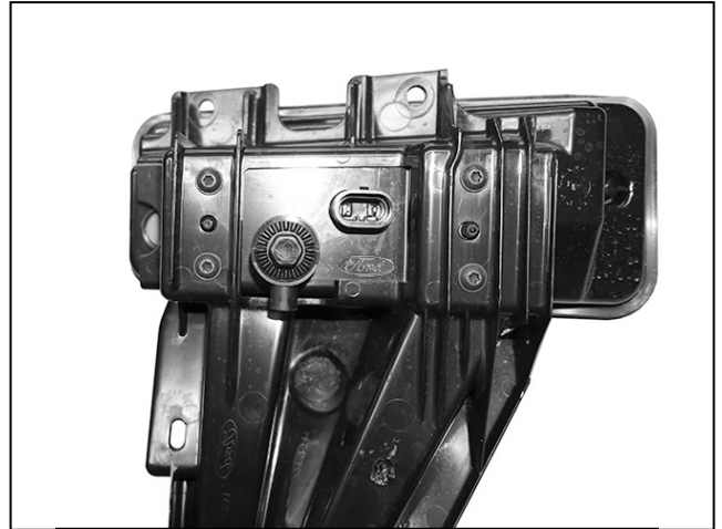
(Fig 21) Remove screws to remove narrow LED fog light from plastic mount
