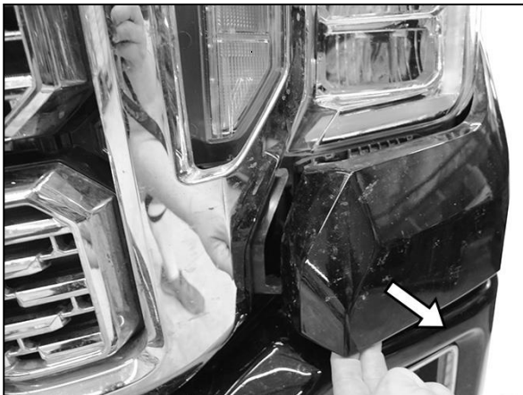
(Fig 1) Pull end of plastic panel (fascia) out and away from grille. Do not remove panel, only release the end of panel covering grille
