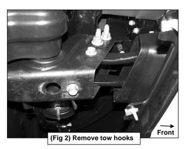
**WARNING!** Do not remove bumper bolts unless the bumper is properly supported on blocks or stands or the bumper may fall.
