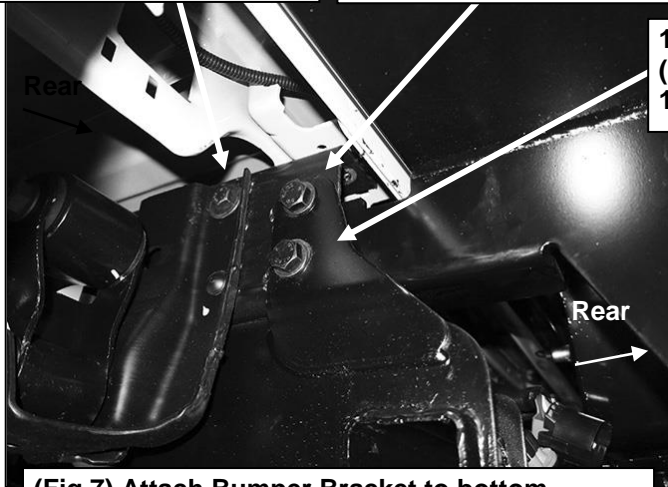
(Fig 7) Attach Bumper Bracket to bottom mounting holes in frame and hitch if equipped
