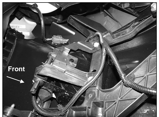
(Fig 4) Unplug lights and sensors if equipped. Unplug harness to bumper and move harness
