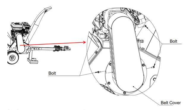
Step 2: Remove the old belts and replace with new belts.
