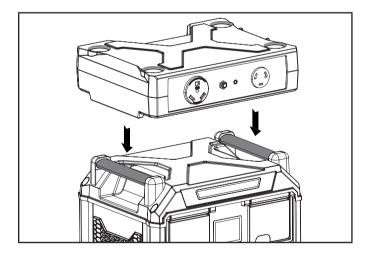
4. Place the second Power Station on top of the parallel kit so that the Power Stations feet fit securely into the slots on top of the parallel kit.
