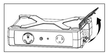
3. Place the parallel kit on top of the heaviest Power Station being paralleled so that the handles on the Power Station fit securely into the slots on the bottom of the parallel kit.
