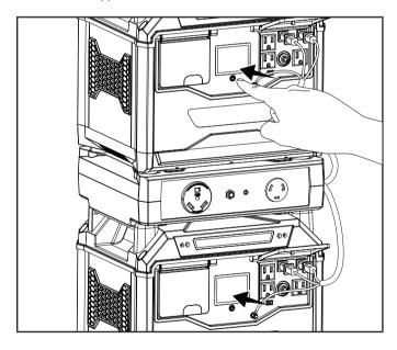
8. Connect devices to the parallel kit and/or Power Stations up to the receptacles' rated amperages. Never exceed the specified rated capacity of the receptacle.
