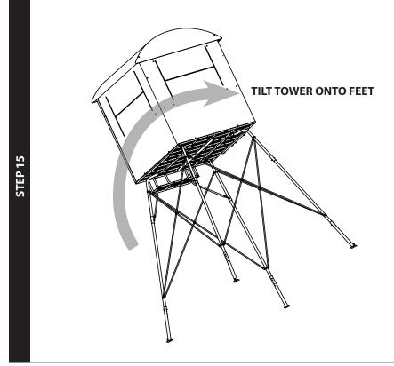
15. With at least four people, carefully lift on the platform side of the tower and tilt onto its feet. **DO NOT** lift only on the blind!
