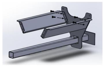
5. Insert 4x Bolts, 8x Washers, and 4x Nuts to secure the Stiffeners to the frame.
