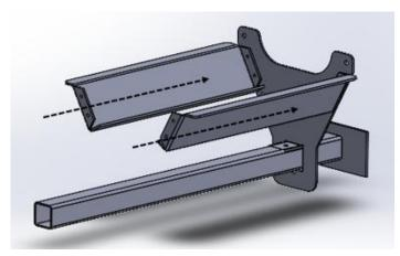
4. Align the 2x Stiffeners to the Front End Frame. For the Small and Large frames, align to the top two holes. For the UV frame, align to the bottom two holes.
