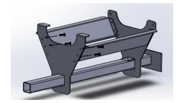
7. Insert 4x Bolts, 8x Washers, and 4x Nuts to secure the Back End Frame to the Stiffeners. Use 1x Bolt to secure Back End Frame onto the hitch attachment.
