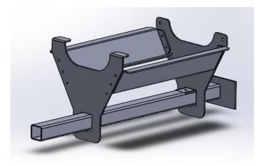
6. Slide the Back End Frame onto the hitch attachment.
