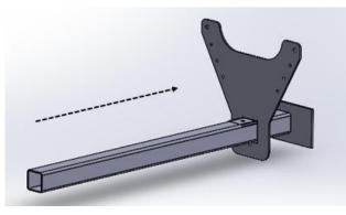
2. Slide 1x Front End Frame onto the hitch attachment
