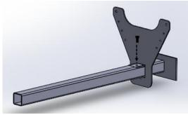
3. Use 1x Bolt to secure the Front End Frame onto the hitch attachment.
