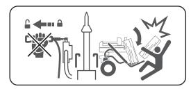
When the wedge is extended and not fully return back, do not pull the control lever outwards, otherwise the log lift table attachment may suddenly drop down, risks of falling the log, damage and injury.
