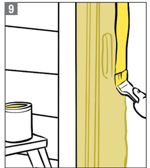
9 Apply additional coats of Liquid over all dried layers.
