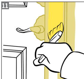
11 Brush Liquid on top of all areas sealed with Paste.
