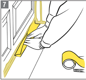
7 Seal door to foundation with Tape, pushing fold into seam.
