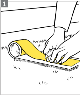
1 Cut Tape to fit opening.
