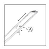
5.Remove the pin A (both sides), adjust height and secure it with cleavis pin.
