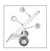
4.Fold up part A and B to the position shown above. Secure cleavis pin at point C as shown above.
