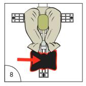
9. Place SANDBAG onto the top of the BACK FOOT to secure the item to the ground.
