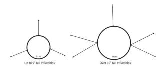
To properly secure your inflatable, install the upper tie downs according to the above graphic. Note that two of the side tie downs must angle forward by at least 30 degrees. Adjust stakes as needed to assure that the inflatable is fully upright and positioned correctly. When the inflatable is correctly positioned and all stakes have been placed, push all of the stakes fully into the ground.
