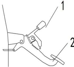
Figure 2-14 Brake pedal 2 and parking brake
