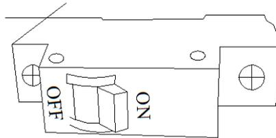
Figure 2-12 Power-off Switch
