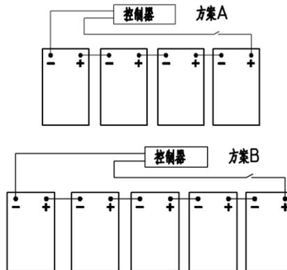
Figure 2-22 Schematic diagram of battery pack wiring
