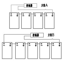
Figure 2-22 Schematic diagram of battery pack wiring
