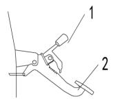
Figure 2-14 Brake pedal 2 and parking brake
