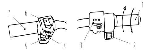
Figure 2-9 Throttle & Function keys 1
