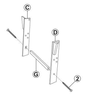
Do not fully tighten hardware until Step 6 is complete.
