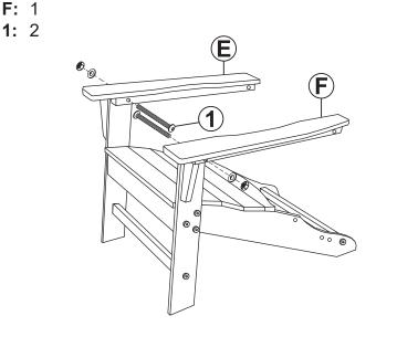
Do not fully tighten hardware until Step 6 is complete.
