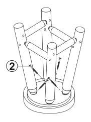
Fasten the legs to the seat using four M3.5x60mm Screws (2).
