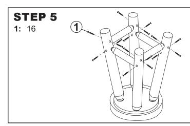
Fasten the footrests to the legs using sixteen M3.5x60mm Screws (1), as shown.
