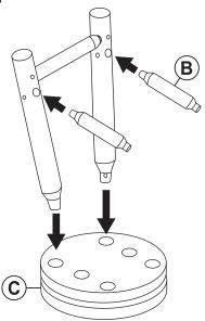
**IMPORTANT:** Ensure the footrest mounting holes are facing the correct direction.
