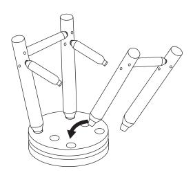
Install the remaining leg set into the seat and align the footrests.
