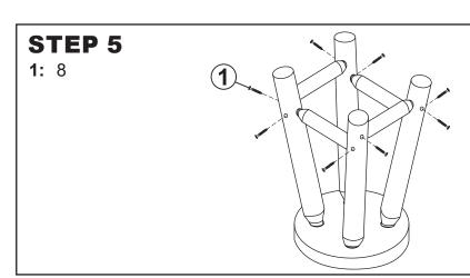
Fasten the footrests to the legs using eight M3.5x60mm Screws (1), as shown.
