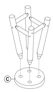
Insert the tops of the four legs into the underside of Seat (C).
