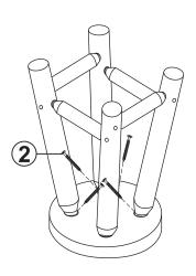
Fasten the legs to the seat using four M3.5x60mm Screws (2).
