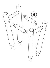
Firmly insert the remaining two Footrests (B) into the upper holes of Legs (A1) and Legs (A2), as shown.
