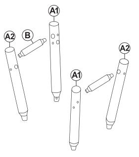
Firmly insert two Support Bar (B) into the lower holes of Legs (A1) and Legs (A2), as shown.
