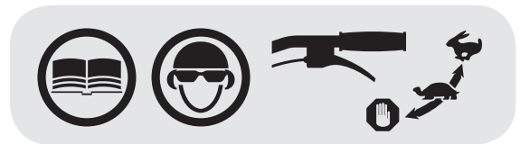
Part No. 10505 SAFETY PRECAUTIONS DECAL - Read entire manual before operating product - Wear eye and hearing protection - Throttle speed control
