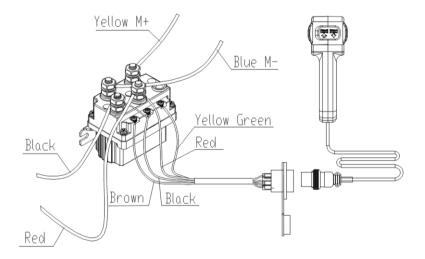
13. Operate the controls briefly to ensure they work properly. If operation is reversed, the power cables may be connected backwards. Correct any such issue before use.
