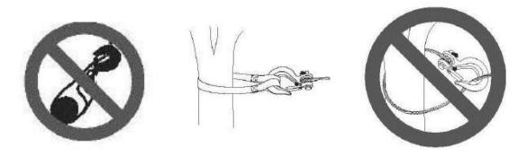
Do not wrap the rope around the object and hook onto the rope itself. This can damage the object being pulled, and kink or fray the rope.
