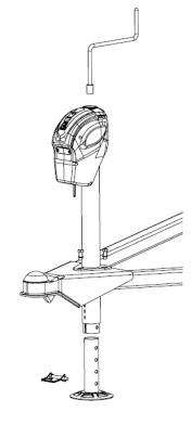
**Note**: Under heavy use, the internal circuit breaker may open, causing the motor to switch off. In this case, release the operating switch, and wait 15 seconds for the breaker to reset before resuming operation.
