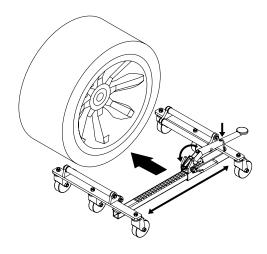
b. Move the Lever to the up position, then pump the Foot Pedal until the tire is just lifted off the ground.
