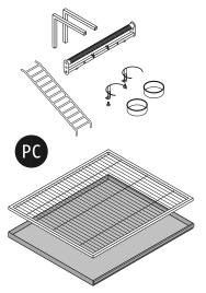
Remove the hex screws from the ends of the perch bar supports. Install the **perch bar** supports on the back panel of the cage.
