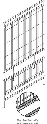
Note: Small loop on the back panel should face the interior. This loop helps hold the bottom grille in place.
