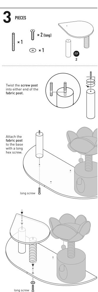
Insert the **leaf platform/short post** unit onto the screw post. Attach the unit to the base with a washer on a
