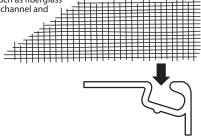
**3.** The flat spline is positioned over the channel.
