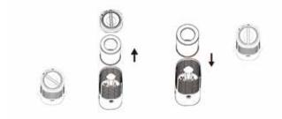
Align the arrow on the cap with OPEN on the unit and screw it in towards the CLOSE position.
