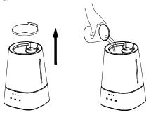
c. Removing the upper cover and taking the water tank off of the base and then filling the water tank with water before returning it to the base.
