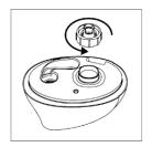
2. Flip over the water tank and open the lid by twisting it to the left
