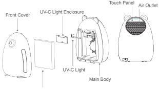
3-in-1 Filter (Carbon Pre-Filter, True HEPA Filter, Antibacterial\* Filter \*Prolongs filter life
