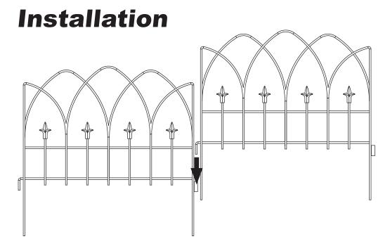
Insert the first fence panel by pushing the legs into the soil.
