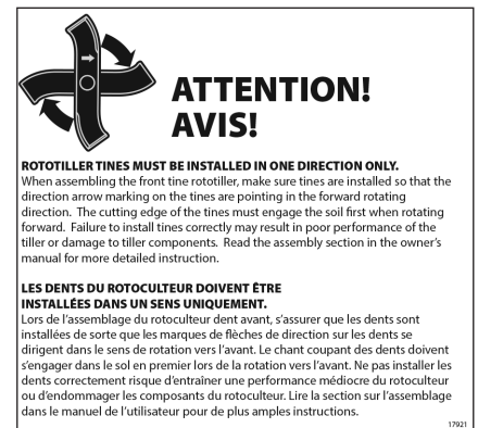
Part No. 17921 CORRECT TINE INSTALLATION
