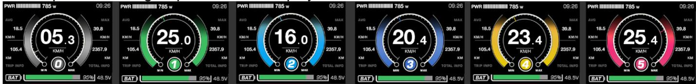
Short press “+” or “-” button to switch assist level. Switching level is not cycled, after reaching 5<sup>th</sup> level, short press “-” button to return to off level. It is the same when adjusting up.
