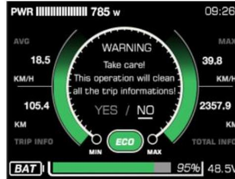
After clearance, the subtotal mileage TRIP is 0, average speed, and max speed is 0. Riding analysis is also 0. ODO information cannot be cleaned manually on the display, professional service tools are required.
