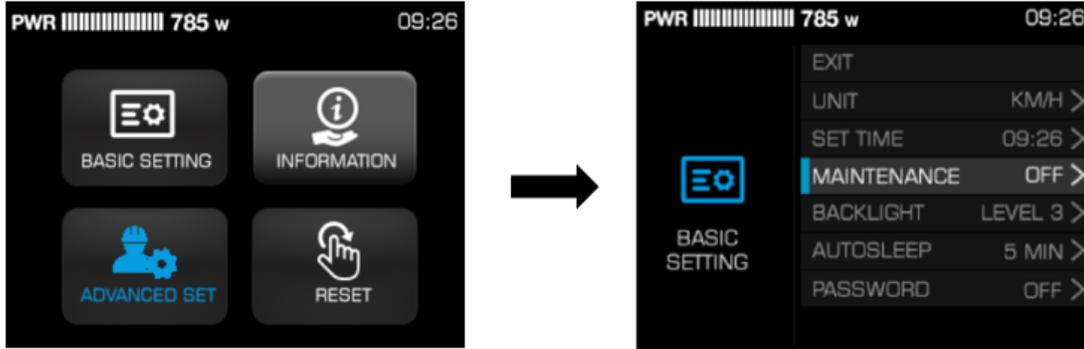
Under any setting interface, short press “M” to enter the next level menu, and long press “M” button to return to the previous level menu.
