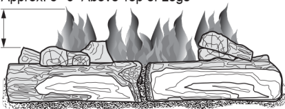
Figure 28 - Correct Burner Flame Pattern
