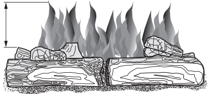
Figure 27 - Incorrect Burner Flame Pattern with Control Knob Set to HI (5)
