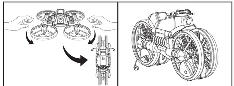
Once you have installed all four wheels, fold the sides of the vehicle inward and connect the wheels to each other. Once folded the bike should be ready to go.
