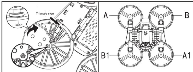
Each blade/wheel has A1, A or B1, B mark. When switching modes, please install the correct one in conjunction to its symbol. To install the wheels, align the triangle mark and the center axis of the main body. Once aligned, install the wheel in the direction of the arrow and align them with the gear.
