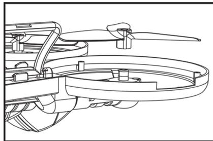
To switch modes from Drone to Bike, make sure the drone is off. Gently pull off the four blades out of the aircraft.
