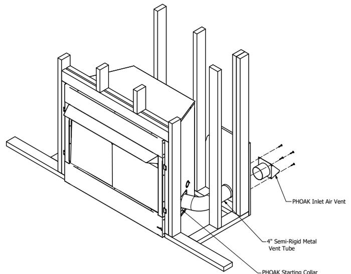
Figure 14 - Simple Outside Air Kit Installation
