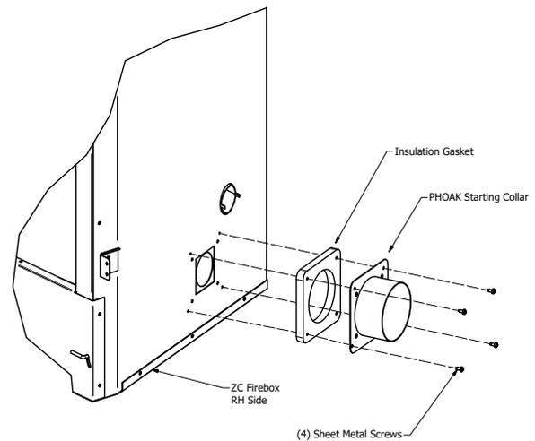
Figure 13 - Outside Air Inlet Collar Attachment
