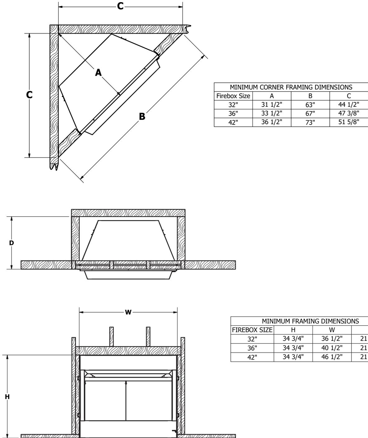
Figure 3 - Framing Dimensions
