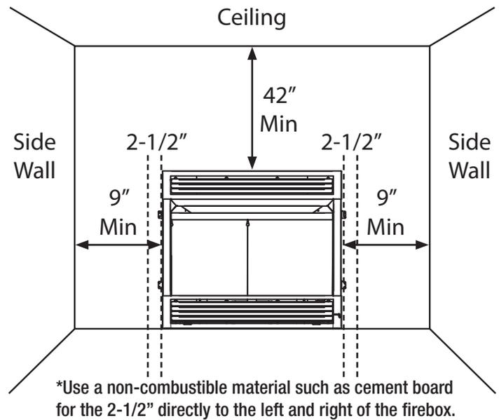
Figure 4 - Clearance to Combustible Surfaces
