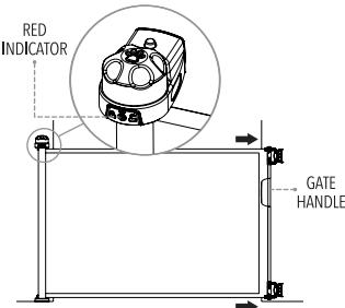
Extend gate by pulling gate handle to handle mounts and hooking onto upper and lower handle mounts. Make sure gate is in unlocked position by checking red indicator window. This will allow gate to open freely.
