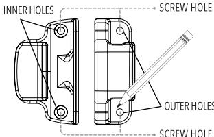
Repeat Step 1 on opposite side of wall using the paper wall mounting template B (I) to help you mark the exact locations to attach the handle mounts.
