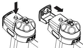
Remove gate by pushing and holding onto circular lock release button while sliding gate outwards from upper mount and upwards from lower mount.
