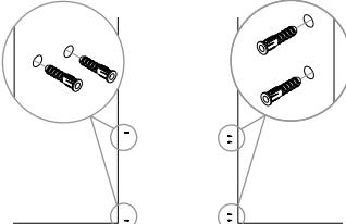
For wall stud surfaces, drill a 1/8" (3mm) hole through guide marks. For drywall surfaces, drill a 1/4" (6mm) hole through guide marks and insert plastic wall anchors.
