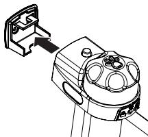
With bottom of gate connected to lower gate mount, push top of gate towards upper gate mount to secure in place.
