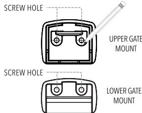
Use the paper wall mounting template A (H) to help you mark the exact locations to attach the gate mounting parts. To use the paper wall mounting template, place it against the wall with the bottom edge of the template touching the floor. You may choose to use a level or measuring device to ensure exact placement. Mark the location of the screw holes of the gate mounting parts through the template and onto the wall.
