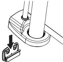
To attach retractable gate (A), align bottom of gate above lower gate mount while sliding downwards.
