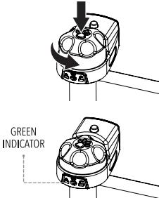
To lock gate in place, push down on upper cap and turn counter-clockwise until stopped. Make sure gate is locked by checking green indicator window. To unlock, turn upper cap clockwise until it pops up.
