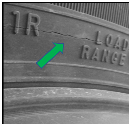
Circumferential Bead Cracking
