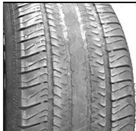
Fast Centerline Wear
