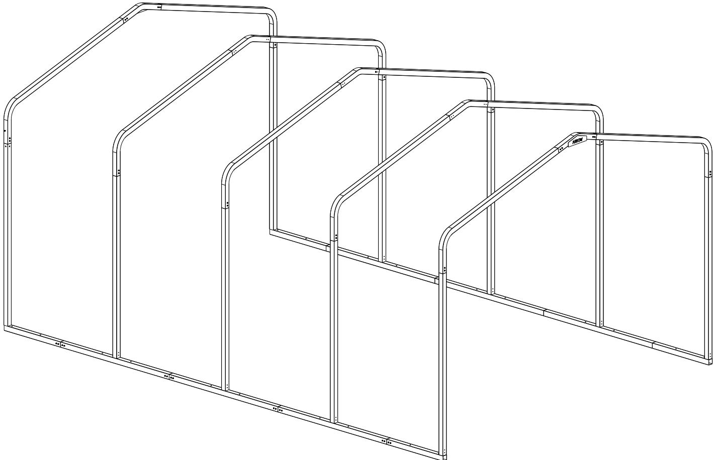
**NOTE:** The 12'W x 20'L x7'H is a base building. Buildings longer than 20' will receive 2 additional boxes for each 4.5', one frame box with 1 middle rib and one panel box with 7 middle panels. These frames and panels are inserted in the middle section of the base building.
