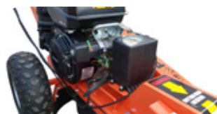
DUAL DIRECT V-BELT 3600 RPM DRIVE
