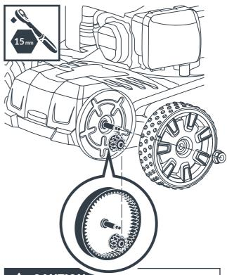
Make ensure the inner gear ring of the wheel and the gear of the wheel guard are meshed in place.
