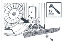
2. Remove the four M6x12 bolts fixing the engine pulley cover and put the engine pulley cover aside.
