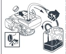
Always keep the air filter and carburetor facing up whenever needed to tip the machine onto its side.
