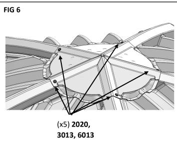
**STEP 6:** Locate roof cap **[04630]**. Align the roof cap over the center of the roof assembly. This step will require standing the roof up to attach it. With the roof on its side, attach the roof cap with the black bolts **[2022]**, rubber washer **[3013]**, and wing nuts **[6013]**. Once all the bolts are in place, tighten down.
