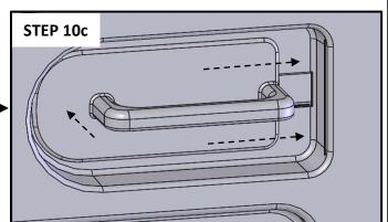
**STEP 10c:** While applying pressure in on the handle to keep the tabs in the slot, slide the handle towards the door frame.
